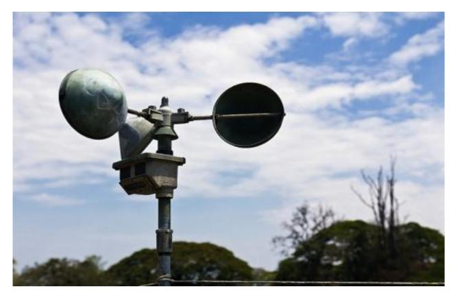
A tool used to measure the speed of wind
